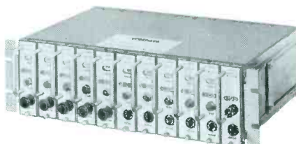
TYPICAL 19 INCH RACK MOUNTING.
